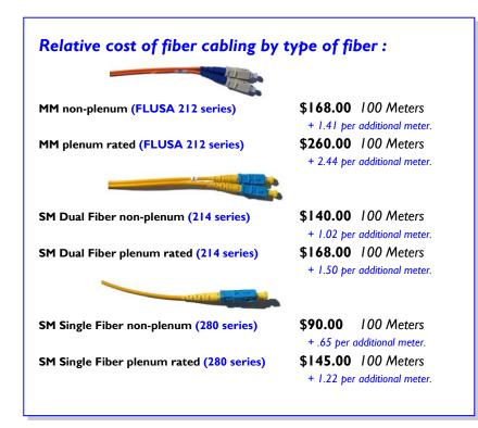
**Note:** Plenum-rated cables are built using a jacketing that is fire-rated for installation in the airspaces (plenums) of buildings. Fire code requires that cables installed in open airflow spaces be plenum-rated so as not to produce toxic fumes in the event of a fire. If the cable is to placed inside a fire-rated conduit, plenum jacketing is typically not required.
